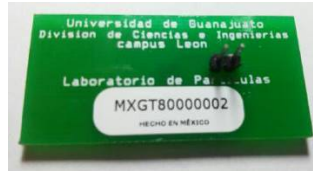
Figure 3 Photodiode board bottom layer.
