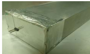
Figure 7 Aluminum block and photodiode isolated optically.
