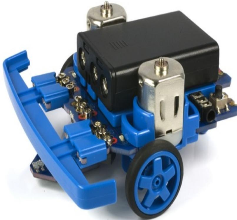
**Fig. 1. Mini robot PICAXE.**
