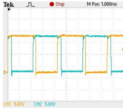
Figure 9 PWM control signals from the TL494 circuit.
