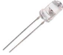
Figura 5 LED ( light-emitting diode ).
