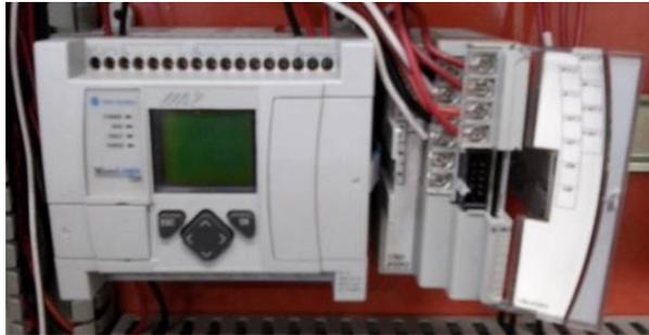
Figura 3 PLC Allen Bradley MicroLogix 1100.
