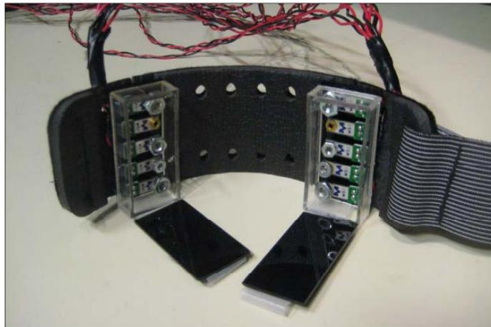
**Fig. 4. Skinput Armband with 10 piezoelectric transducers [6].**
