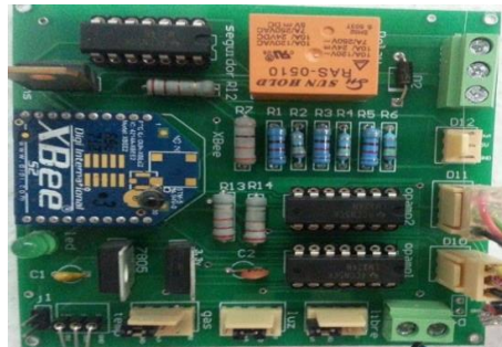
Figure 8 Signal conditioning board.
