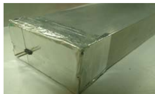
Figure 7 Aluminum block and photodiode isolated optically.
